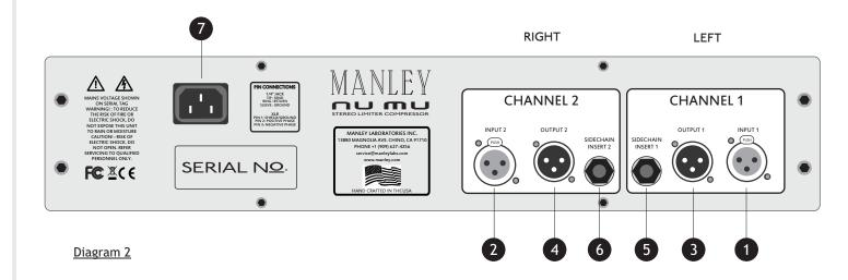
XLR INPUT 1 (TRANSFORMER BALANCED) (CH1, LEFT) PIN 1: GROUND PIN 2: (+) PIN 3: (-) XLR INPUT 2 (TRANSFORMER BALANCED) (CH2, RIGHT) PIN 1: GROUND PIN 2: (+) PIN 3: (-) XLR OUTPUT 1 (IMPEDANCE BALANCED) (CH1, LEFT) PIN 1: GROUND PIN 2: (+) PIN 3: (-) XLR OUTPUT 2 (IMPEDANCE BALANCED) (CH2, RIGHT) PIN 1: GROUND PIN 2: (+) PIN 3: (-)
