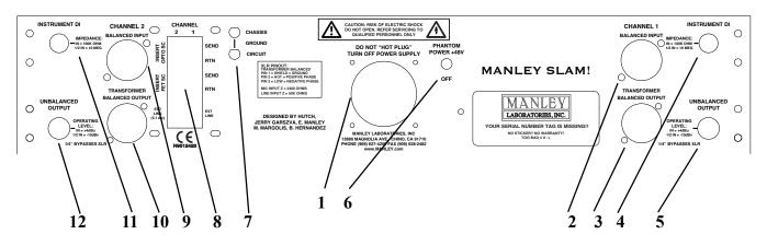
This is just a description of the various jacks and switches on the back. We suggest that you might want to not rack-mount the SLAM! until you've spent some time becoming familiar with the various patching and switches. Sorry, but the back panel is more complex than most gear and there are options galore. That's what happens when you get what everybody asks for. For simple maps that show a few examples of how to patch the SLAM!, check out Page
