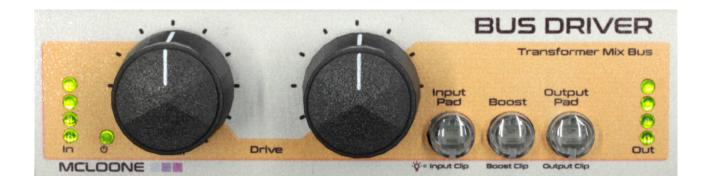
**Input Pad** - Switches a reduction of around -30dB. Use this when connecting to equipment which has a +19dBu or +22dBu output level, to avoid distortion.
