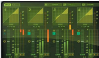
**X-Over** – crossover points are graphically adjustable. A dynamic plot of the input, output, or overall dynamics action (Gate+Expander+Compressor) can be displayed, and is updated alongside any crossover adjustments. The band gain sliders are moved up next to the IO curves for the Gate, Expander, and Compressor.
