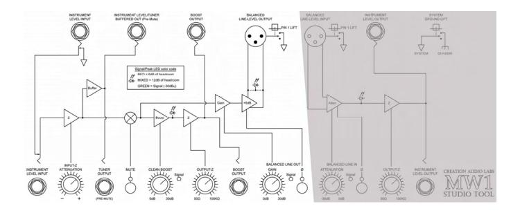
\*\*\*All ¼" jacks are duplicated on the front and back of the MW1 Studio Tool. With the exception of the **INSTRUMENT LEVEL INPUT** connections, all ¼" jacks front and back will be active at the same time. As such, the duality of the output jacks allows for multiple signal path routing. The **front** INSTRUMENT LEVEL INPUT takes priority over the rear input.
