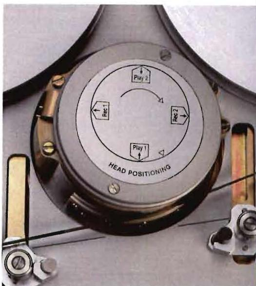
*The scanner is equipped with four heads, two for recording and two for playback. This advanced technology gives an improvement in signal level compared to stationary head formats, and allows full confidence playback.*
