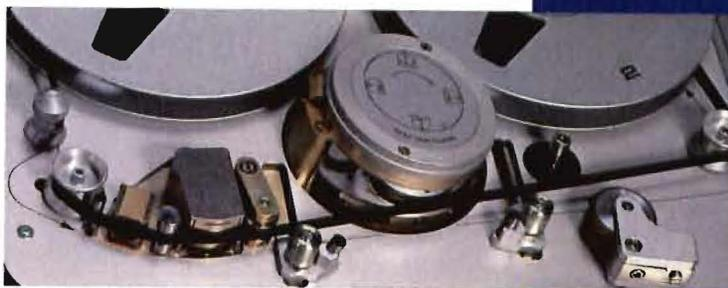
*The rugged, open reel NAGRA-D format gives you easy access to the tape transport mechanism. Visual checking, cleaning, and rough scissor editing are possible.*
