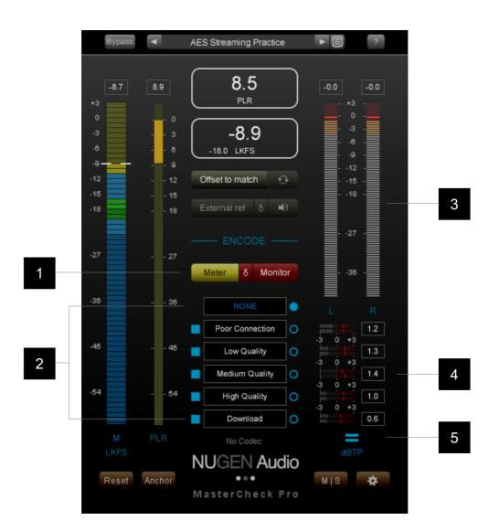
**1 Metering and Monitoring.** These controls determine the output metering and monitoring for MasterCheck pro.
