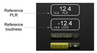
Place MasterCheck as you usually would to monitor your mix and click the 'External ref.' button. If you are using more than one NUGEN Audio SEND plug-in in your mix, you may need to open the settings panel and select the correct source from the drop down menu.
