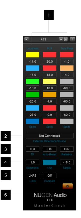
1 **Colour Splits.** The colour splits can be used to define different zones within the bar meters, to indicate desired targets/out of specification values etc. The split values determine the position of the colour boundaries. Click-drag up and down to change the value or double click to enter a specific value. To change the colours of the sections, click the swatch to open the colour picker window.
