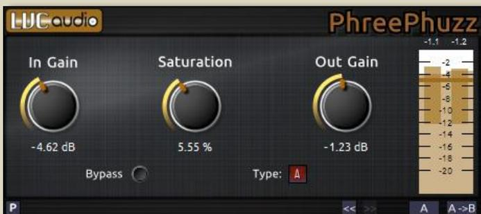
The main interface for PhreePhuzz is very simple. It includes three knobs for altering the saturation and gain. Additionally, there is a bypass switch, selector switch for the saturation types, and a preset import/export button.
