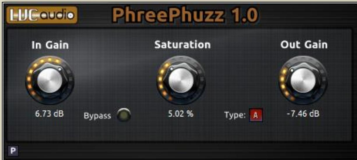
**Button and Selector Features:** The main controls of PhreePhuzz are adjusted by using various knobs and buttons. For buttons such as Bypass or Solo, clicking the button one time will enable the feature. Clicking a second time will disable the feature. Some buttons, such as Oversample, contain more than two different settings (i.e., more than on and off). Each click of the button will cycle the control through all of its settings.
